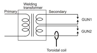
Current of only one circuit is kept constant in this case.
