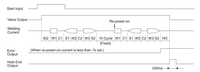
• The power is turned on again when the welding current is less than -% set or no power is turned on.
