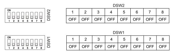
Note: Please do not set dip switch during power "ON". Dip switch should be set during power "OFF".
