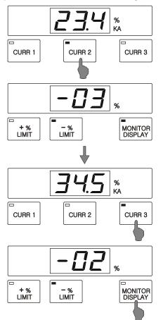
After welding, the measured current and ±% is displayed. When push a selection button (among Curr1, 2, 3) during monitor display LED is illuminated, the selected "Current" is illuminated and display the measured welding current.
