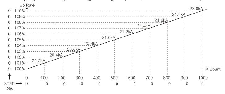
• 9 stepper (When DSW1-(4) is turned off)\_It is working as step No. 0~9.
